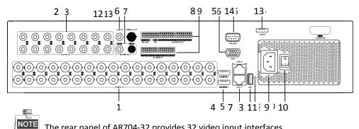
The rear panel of AR704-32 provides 32 video input interfaces.
